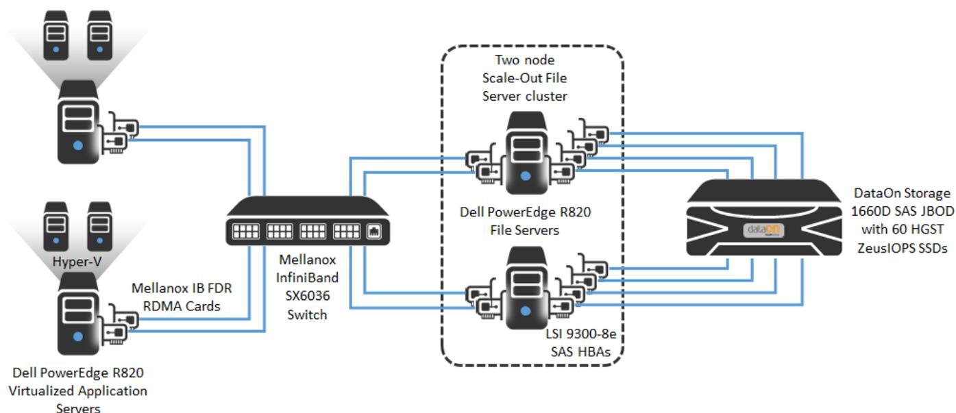
Multiple steps were required from a server, storage, and network standpoint to enable a highly performing Scale-Out File Server platform. From a server standpoint, the SOFS is built on top of a Windows Server Failover Cluster. The top picture in Figure 4 shows a snapshot of Failover Cluster Manager where a two-node failover cluster was created. Next, the SOFS role was added to the failover cluster, which finished the cluster creation.
