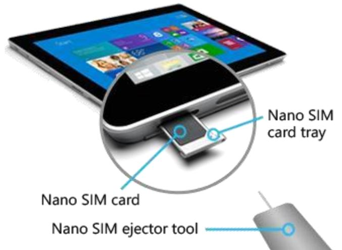
If you have a Surface 3 Type Cover, click it into place and open the kickstand. If you have a Surface 3 (4G LTE) and an uninstalled Nano SIM card, install the SIM card.
