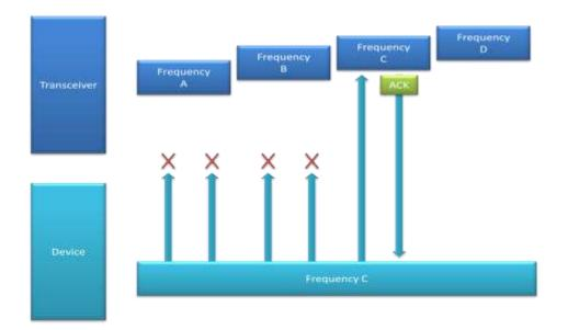
The transceiver and peripheral connect the same way when they are initially installed and the user first presses a key or moves the mouse. The transceiver locks on to the peripheral almost immediately, with no need for human intervention.
