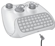
To connect a headset, plug the headset's connector into the 2.5-mm connector jack on Chatpad.
