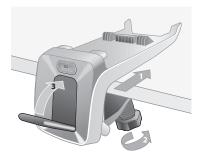
To move the clamp to another location, pull the quick-release lever, loosen the screw, and slide the clamp off the table.
