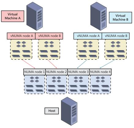
FIGURE 2-9 Example of virtual NUMA at work.
