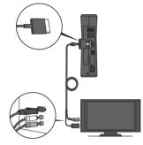
Thanks for choosing the Xbox  $360^{\circ}$  VGA HD AV Cable to connect your Xbox 360 console to your VGA CRT, LCD, or HDTV monitor, including PC monitors. The cable also connects to analog audio amplifiers. It is for use exclusively with the Xbox 360 video game and entertainment system.
