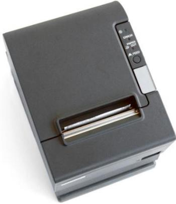
**Point-of-Sale Printer** This concept device was created by wedding a serial point-of-sale printer to a Freescale i.MXS development board, which serves as a gateway to network-enable the printer using Devices Profile for Web Services (DPWS) protocols. DPWS allows terminals to discover the printer on the network and promises wider compatibility with retail POS equipment from different vendors.
