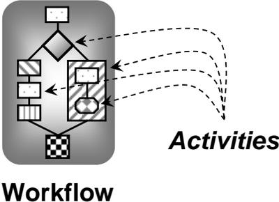
WWF ships with a set of general purpose activities for defining workflows. This *base activity library* provides the ability to define control flows using familiar constructs such as if/else and while loops. It also includes a rules engine, support for communicating with other software using web services, and more.
