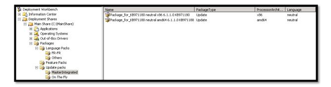
At this time, you do not have Os packages in the **On The Fly** folder. This is because the next step is to create the Reference image. The Reference Image must be up to date when you create it.
